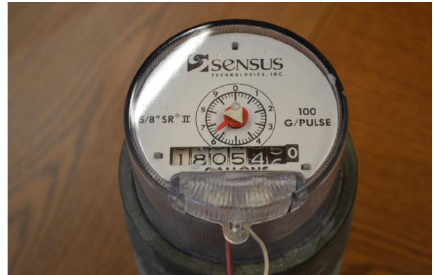
A Sensus Meter. There is no black box attached to this meter so it is not read by a radio, it is manually read by a city meter reader. The white triangle is a leak indicator, it indicates use. This meter reads 1,805 gallons
